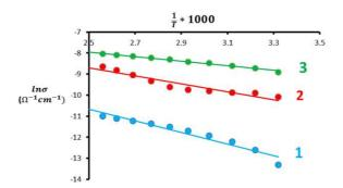
Figure 9: The Relation between in σ and Reciprocal Temperature for the Complex(1), the Complex Doped with DDQ(2) and Iodine Doped(3)
