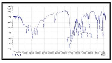
Figure 2: IR Spectrum of PcCo(II)
