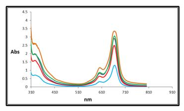
Figure 4: Variation of Absorbance with Concentration of the Complex PcCo (II). Blue Line (Lower Line) is of Lower Concentration and the Brown Line (Upper Line) is of the Higher Concentration
