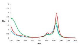
Figure 5: The Shift of  $\lambda_{max}$  for both Iodine-Complex and DDQ-Complex Solutions in DMF
