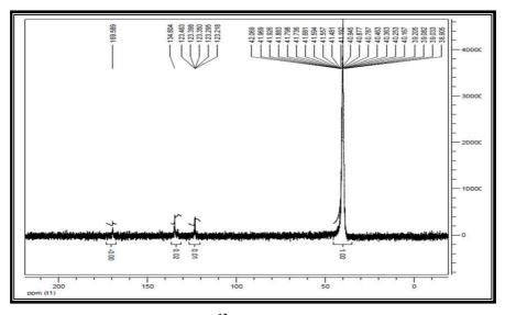
Figure 7: The <sup>13</sup>C Spectrum of PcCo(II)
