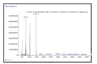
Figure 10: The Mas Spectrum of PcCo (II)
