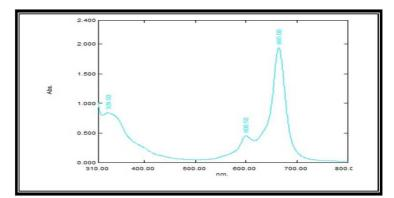
Figure 3: The Electronic Spectrum of PcCo (II) in DMF
